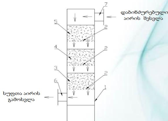
1-building; 2-holding the grid; 3,4-modified sorbent layer; 5-gas running layer; Output of 6-pure gas; 7-contaminated gas entrance.
