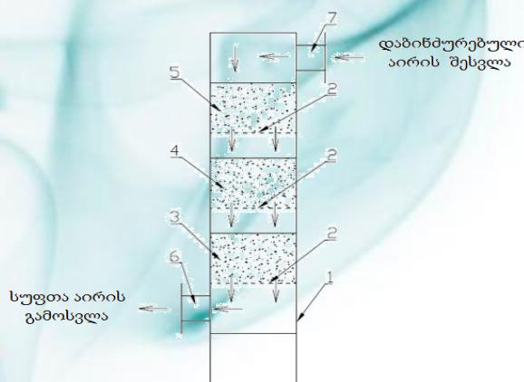
1-building; 2-holding the grid; 3,4-modified sorbent layer; 5-gas running layer; Output of 6-pure gas; 7-contaminated gas entrance.
